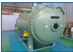
Sewage Treatment Plant (5.4kg-O 3 /h)
