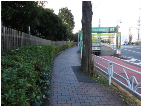
Figure 3.3 Example of Physical Separation Provided between Roadways and Sidewalks
