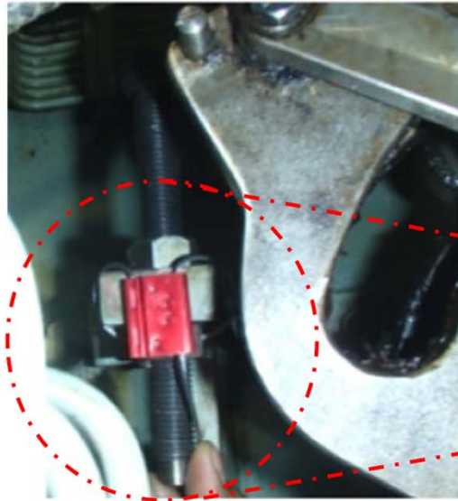
Mechanical stop screw sealed by wire
