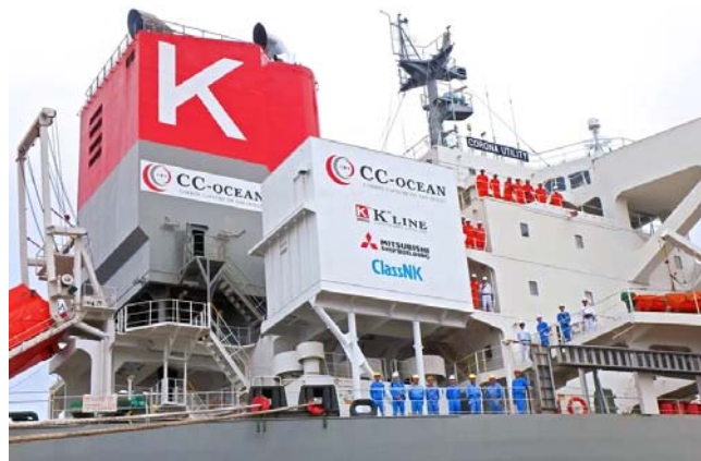
Figure 5.3-1: Project by Mitsubishi Shipbuilding, Kawasaki Kisen Kaisha, and ClassNK View of the CO 2 capture system that has been installed on board the ship
